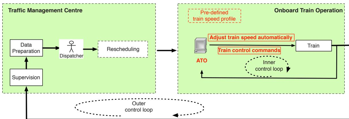
Figure 6 – Optimisation with the Automatic Train Operation (ATO).
