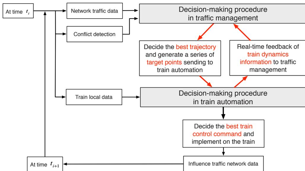
Figure 8 – The highlights in the integrated optimisation model: the decision-making procedure and the bidirectional communication between traffic management and train automation.
