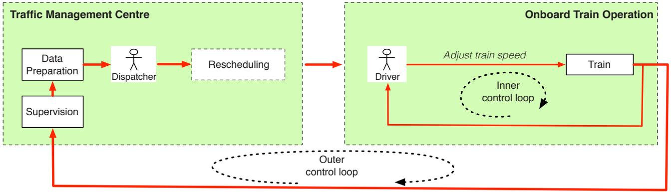
Figure 1 – Non-optimised railway operation depending on the expertise of the dispatcher and the driver.
