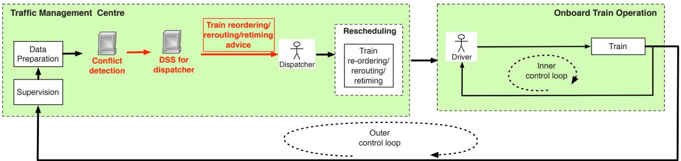
Figure 3 – Optimisation with the Decision Support System (DSS) for dispatchers.
