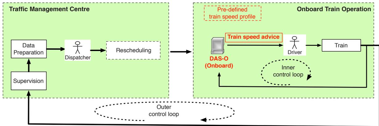
Figure 5 – Optimisation with Driver Advisory System - Onboard (DAS-O).
