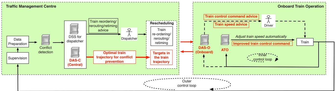
Figure 7 – The integrated optimisation model combining optimisation schemes of DSS, DAS-C, DAS-O and ATO.
