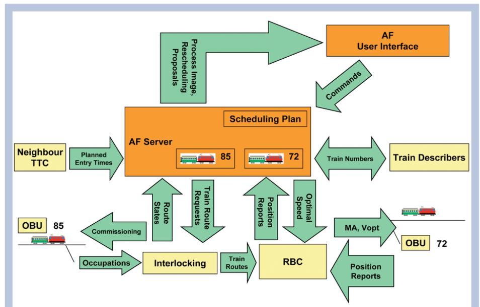
Fig. 1: Operations control system, ETCS Level 2, in the Lötschberg Base Tunnel
